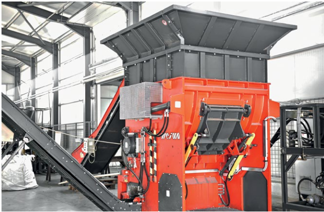
WEIMA W5.18 with wide inspection flap for the maintenance or removal of any impurities
