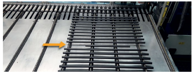
The new SawControl module, developed by PIXARGUS, makes profile cutting an integrated element of quality control. The software module performs two control functions for the cutting device: It sets the regular spacing for the continuous cutting process and cuts out defective profile portions at short lengths (Picture © COOPER Standard)
