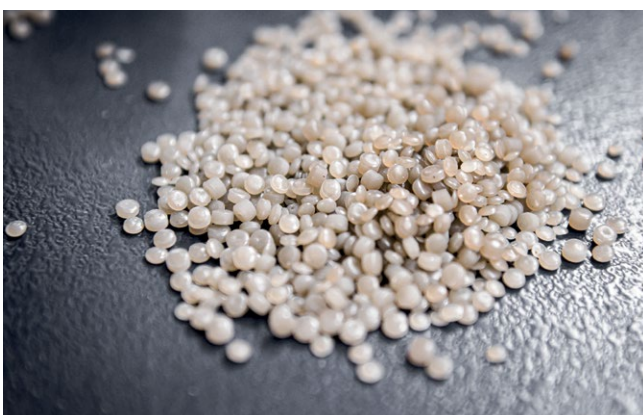
High-quality regranulates at the end of the recycling line
