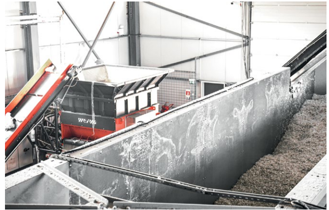
First step: The plastic shredder processes a wide range of materials into homogeneous flake sizes
